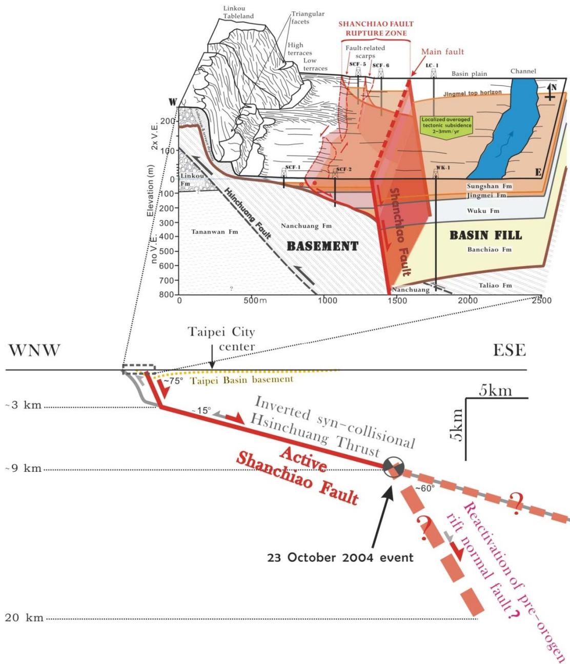
Figure illustrating the structure of the Shanchiao Fault at near surface level and crustal scale.
